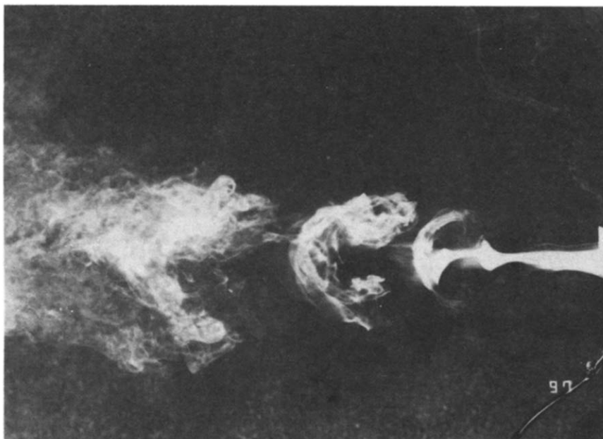
FIG. 2. Typical jet flow structure for Re = 2500 and b = 20 mm.
